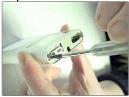
Use the included Phillips screwdriver to remove the two screws at the top of the iPod, as shown. Set the screws aside for reassembly. **PLEASE NOTE: Your tools may look different than those pictured.**
