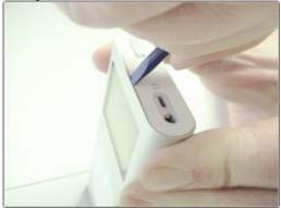
Using the included flathead screwdriver, CAREFULLY pry off the white plastic top of the iPod Mini. It may help to note that SLIGHTLY squeezing the sides of the device can create more space between the white plastic piece and the metal case. It also helps to press toward the metal case rather than the plastic. The white top may be attached with glue.
