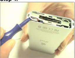
Use the plastic screwdriver to pry each corner of the metal piece at the bottom of the iPod, as shown, until the entire piece comes off. Set it aside for reassembly. Step 5.
