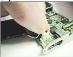
Disconnect the old battery from the iPod by GENTLY pulling upward on the connector with your thumb and forefinger, as shown, or with tweezers. Do not pull on the wires, only pull on the white connector piece to avoid breaking the wires from the connector. Also, use a finger from your other hand to brace the ivory colored part of the connector which is permanently attached to the green motherboard to avoid damaging the connector seat.
