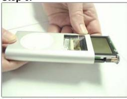
Press from the bottom of the iPod to slide the motherboard out of the iPod casing through the top, as shown. Keep the pressure as even as possible – don't press on only one side. If the motherboard seems stuck, DO NOT apply more pressure. Instead, try jiggling it a little as you press upward.
