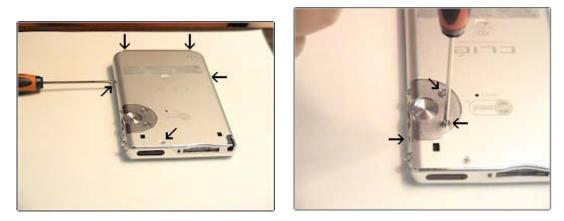
Make certain to replace all eight screws you removed previously. FULLY CHARGE your new battery before use. (Allow at least three hours. For quality control, we pre-charge many of our batteries, so yours may require less time.)
