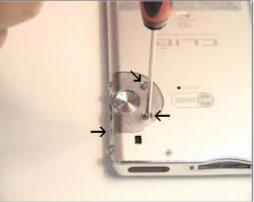
Remove the three screws around the scroll wheel cover, as shown. Set the screws aside for reassembly.
