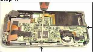
Remove the two screws on the motherboard, as shown, to access the battery. Set the screws aside for reassembly. Make sure to keep track of which screws belong with the motherboard.
