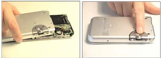
Slide the back cover of the PDA back on from the bottom, then put on the scroll wheel cover.
