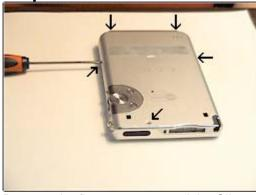
Remove the five screws around the Clie, as shown, using the included Phillips screwdriver. (Your tool may look different than the picture.) Set the screws aside for reassembly.
