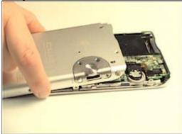
Once the screws have been removed, GENTLY remove the scroll wheel cover and back cover of the Clie by lifting them off, as shown. Use the plastic flathead screwdriver to assist as needed.
