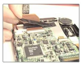
Replace the motherboard screws as shown above, plus the ribbon cable clamp, and the black protective tape over the ribbon cable clamp as shown (if applicable) and the tape over the power cable connectors, as shown.
