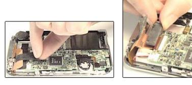
There will be a piece of black tape covering the power cable connectors. Gently lift it using your thumb and forefinger to expose them, taking care not to damage or sever the tape or cables. Then gently remove the clamp that connects the ribbon cable by pulling upward, as shown. If it is taped down, remove the tape.
