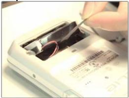
Lift the main body of the battery out by pulling upward on the grey cloth tab, as shown. Leave the connector plugged in for this step.
