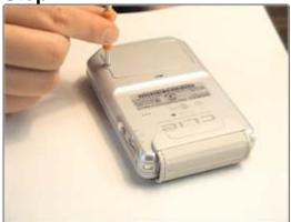
Remove the screw on the battery compartment, as shown, using the included Phillips screwdriver. (Your tool may look different than the picture shown.) Set the screw aside for reassembly.
