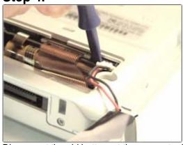
Disconnect the old battery at the connector by placing the plastic flathead screwdriver on one side of the connector and twisting until that side comes out, then pull outward on the connector with your thumb and forefinger or tweezers. Be very sure that you are pulling outward on only the part of the connector that comes out, NOT on the whole connector.
