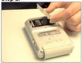
Remove the battery compartment cover. Set the cover aside for reassembly.
