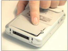
Replace the battery compartment cover and the screw. FULLY CHARGE your new battery before use. (Allow at least three hours. For quality control, we pre-charge many of our batteries, so yours may require less time.)
