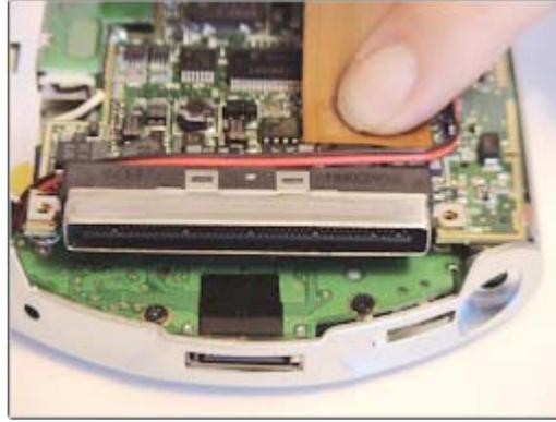
There may be a small piece of protective tape covering the connector on the new battery. Remove the tape before proceeding. Making sure that your battery is facing the right direction (connector towards the bottom of the iPaq), connect the new battery by pressing the connector at the end of the ribbon cable into the socket as shown. Do not press too hard or try to force the pieces together. They will fit easily when correctly aligned.
