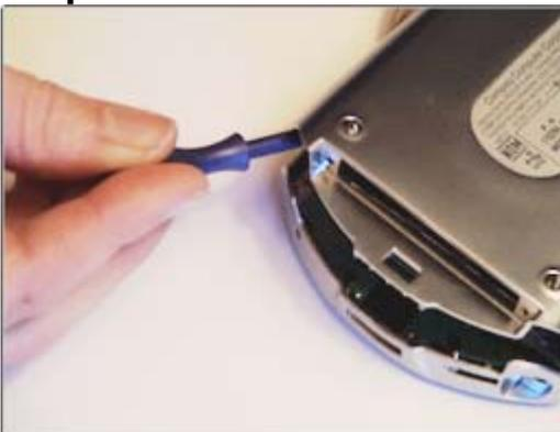
Pry around the edges of the iPaq until the cover pops open. When this occurs, do not immediately pull the cover all the way off, as the old battery will still be connected to your iPaq by a yellow circuit cable. The battery should be glued to the back of the iPaq case.
