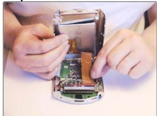
Disconnect the old battery at the connector by CAREFULLY pulling upward on the ribbon near the connector with your thumb and forefinger.
