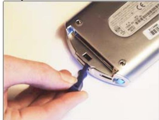
Once the screws have been removed, GENTLY pry open the iPaq case (starting at the bottom, as shown) using the included plastic screwdriver or any small flathead screwdriver. Be very careful, but keep in mind that the iPaq battery cover is glued on. Some resistance is normal.
