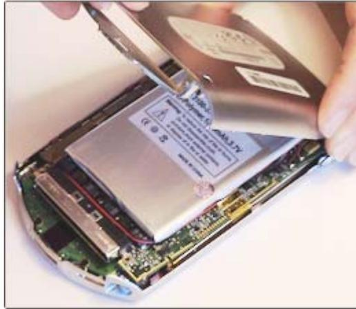
Remove the old battery from the back of the iPaq case, using a screwdriver to pry it out if necessary. Take care not to break the old battery while removing it. Press the back cover of the iPaq on over the new battery and screw the four screws back in. **FULLY CHARGE** your new battery before use. (Allow at least three hours. For quality control, we pre-charge many of our batteries, so yours may require less time.)
