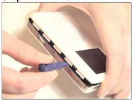
CAREFULLY pry open the entire iPod case, moving around the iPod from your starting point. You will need to use the pry tool to unclip each white clip by pressing it gently inward and then twisting.
