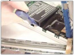
Once the wires are free, use your fingers or the flathead screwdriver to VERY GENTLY remove the old battery. It will be glued in, but be extremely careful not to damage the battery or the circuits beneath it when prying it free. Start at the corners to avoid contact with or damage to the circuits beneath the battery.
