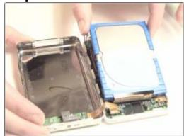
When the iPod case is unclipped, hold the hard drive (it is surrounded by blue plastic) as you separate/open but **DO NOT completely disconnect** the back case of the iPod. The back case should remain connected to the iPod by its connector cable throughout the battery replacement process.
