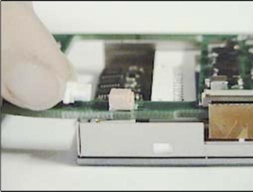
Disconnect the old battery at the connector by CAREFULLY pulling outward on the connector with your thumb and forefinger. Be very sure that you are pulling outward on only the part of the connector that comes out, as shown, NOT on the whole connector.
