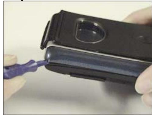
Once the screws have been removed, GENTLY pry open the Palm case (starting at either top corner, as shown) using the included plastic screwdriver or any small flathead screwdriver. Pry all around the device until the front cover comes open completely, but **DO NOT** remove it yet.
