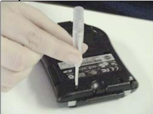
Remove the four screws on the back of the PDA. They will be either T5 or T6 Torx screws. We include both screwdriver sizes. First try removing the screws using the included Torx T6 screwdriver (clear handle). If it is the wrong size, then use the T5 (blue handle). It is important to try the T6 first to avoid stripping the screws. Set the screws aside for reassembly.
