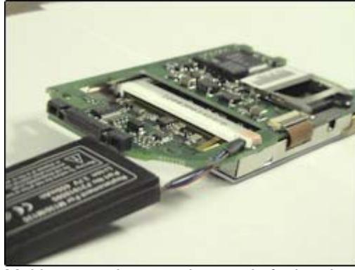
Making sure that your battery is facing the right direction (ribbon cable towards the connector), connect the new battery by pressing the connector at the end of the ribbon cable into the socket as shown. Note the location of the prongs in the socket of the Palm and the location of the plugs for the prongs on the battery connector, and connect them accordingly. Do not press too hard or try to force the pieces together. They will fit easily when correctly aligned.
