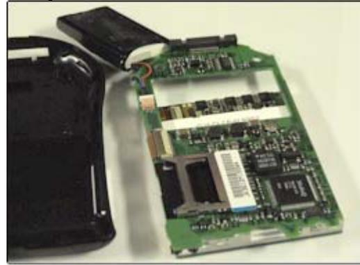
Remove the pull tab at the back of the Palm, then remove the motherboard from the back case and flip it so you see the battery connector, as shown. If the motherboard does not come out easily, try pressing upward from the port at the bottom of the palm. The power port connector is attached to the motherboard, but can get stuck to the back case.
