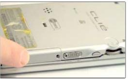
Replace the back of the Clie and screw the five screws back in from **step 2**. Replace the battery compartment cover and screw from **step 1**. FULLY CHARGE your new battery before use. (Allow at least three hours. For quality control, we precharge many of our batteries, so yours may require less time.)
