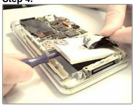
Remove your old battery from its seat, using the plastic flathead screwdriver if needed. Leave the connector plugged in for this step. The battery may be glued or taped in, so remove the tape or pry under the battery GENTLY until it comes loose. Take care not to break the old battery.
