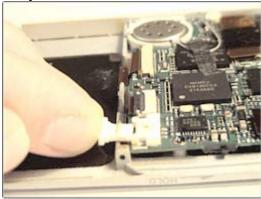
Disconnect the old battery at the connector by CAREFULLY pulling outward on the connector with your thumb and forefinger. Be very sure that you are pulling outward on only the part of the connector that comes out, as shown.
