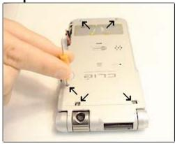
Remove the five screws around the back of the Clie, as shown, using the included Phillips screwdriver. (Your model may have four screws and require a small flathead screwdriver, which we have also included.) Set the screws aside for reassembly.
