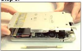
Once the screws have been removed, GENTLY pry or lift the back cover off, as shown.
