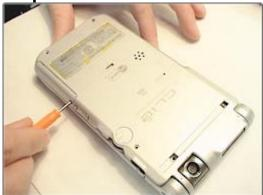
Remove the one screw on the battery compartment using the included Phillips screwdriver, as shown, then the cover itself. Set them aside for reassembly. Do not attempt to remove the battery yet.
